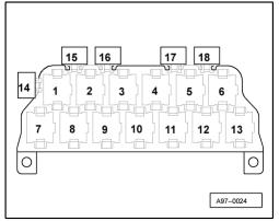
Relay positions 11 - Starter inhibitor relay (J207)
