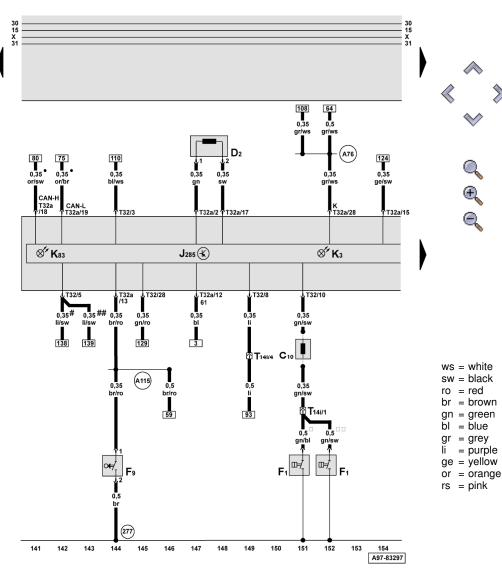
Dash panel insert, handbrake warning switch, oil pressure switch, immobilizer C10 - Suppression filter
