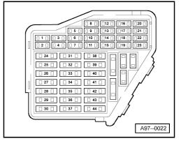
From fuse number 23 upwards the fuses in the fuse box are designated as 223 etc. in the Current Flow Diagram.
